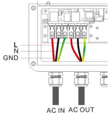
③ Connect the AC output line properly according to the cable sequence and terminal position shown in the above figure. Please connect the ground wire first, then the live wire and the neutral wire.
