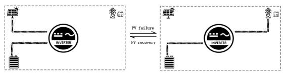
**2. Mains First:** priority shall be given to charging by Mains Power, and charging with PV power will be started only when the Mains has failed.
