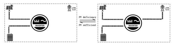
**4. Only Solar:** Only PV charging, no mains charging is initiated. This is the most energy-efficient mode and the battery power comes from solar energy, which is usually used in regions with good daylighting conditions.
