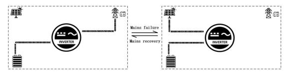
**3. Hybrid Charging:** hybrid charging of PV and Mains Power, give priority to PV MPPT charging, and supplement Mains Power when PV energy is insufficient. When the PV energy is sufficient, the Mains Power will stop charging. This is the mode of fast charging and suitable for unstable areas of power grid, and can provide sufficient backup power at any time.
