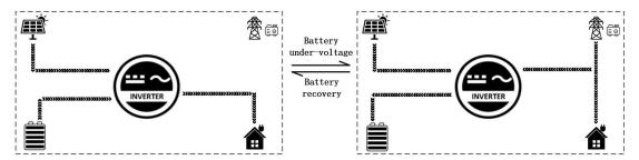
4. Hybrid Function: when the battery is not connected or fully charged, the load is powered with the hybrid of PV and Mains Power, with the maximum output power of PV output.
