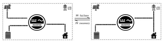
2. Mains First: switch to inverter power supply only when Mains Power has failed, which is equivalent to backup UPS and is used in regions with unstable power grid.
