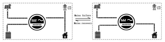
**3. Inverter First:** switch to Mains Power supply only when the battery is under-voltage. This mode uses DC energy to the maximum extent and is used in regions with stable power grid.
