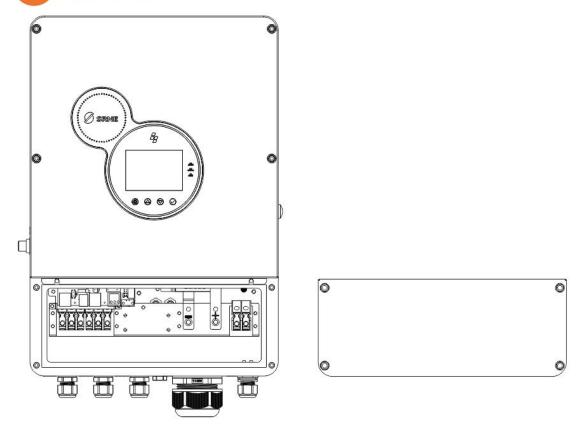
Step 5: Connect the Wire. (Note: The wire shall penetrate into the corresponding joint before crimping the terminal.)
