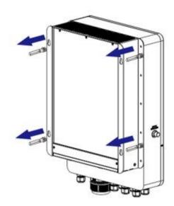
Step 4: Remove the terminal protection cover.
