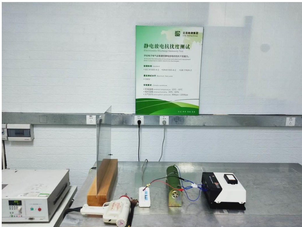
Test Setup Photo of Electrostatic Discharge Test
