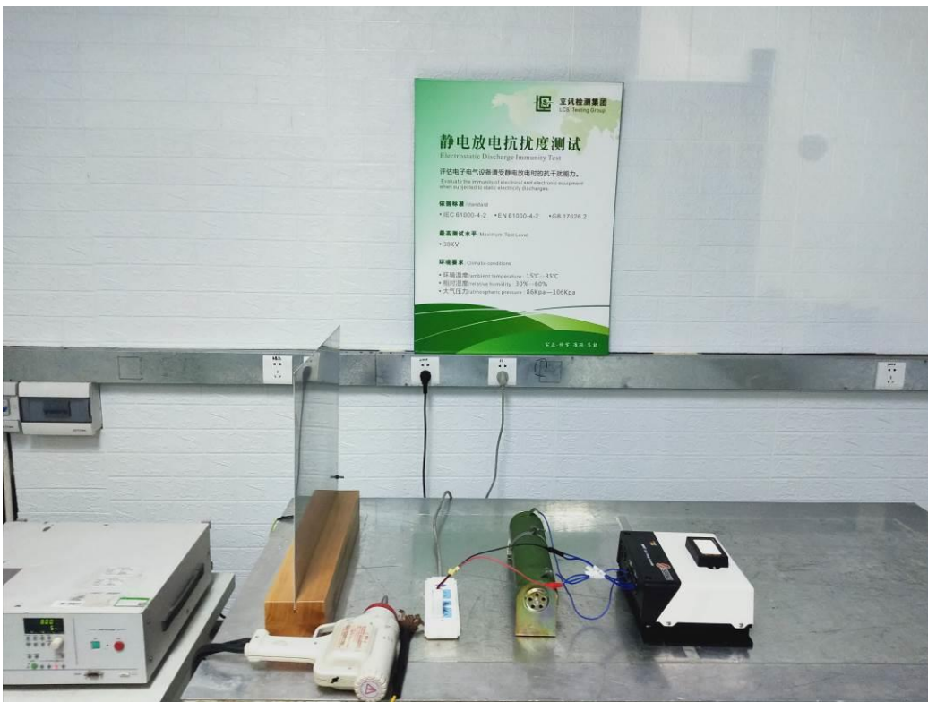
Test Setup Photo of Electrostatic Discharge Test
