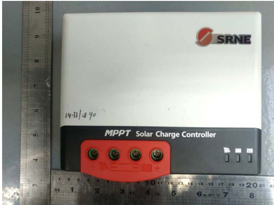
MC2440N10# front view of the BCC
