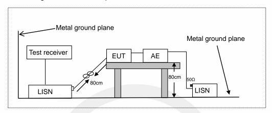
LISN: Line Impedance Stabilization Network
